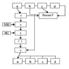
Fig 1:-One MD5 iteration
